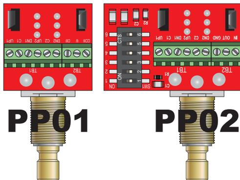
**P**ush/pull pots should be viewed as two separate devices - a pot plus a switch - that share a common architecture. You treat the two elements separately, so the pot portion does one thing, and the switch portion does something else.
