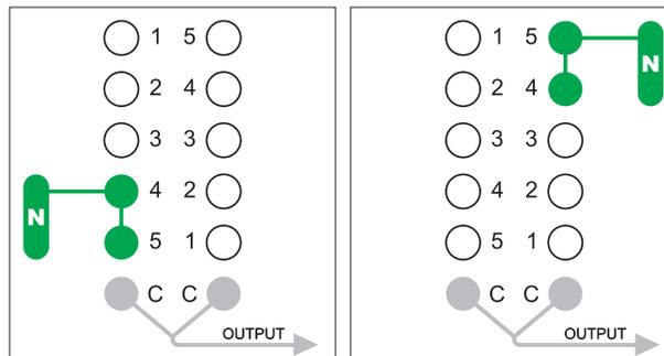
The pickup's ground wire would go to ground, of course. But the hot wire is connected to lugs 4 and 5, so the pickup will come on in positions 4 and 5, so
