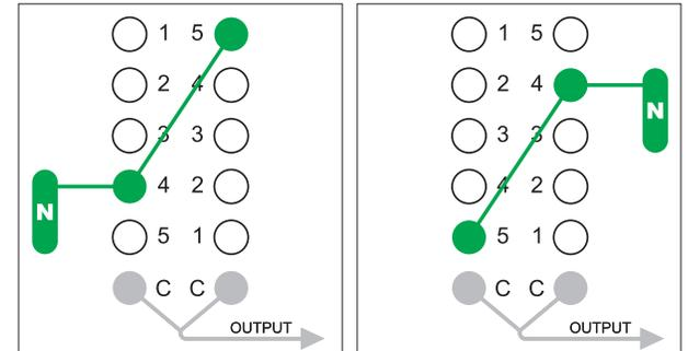
In any of these four connection schemes, the neck pickup will come on in positions 4 and 5. Simple!
