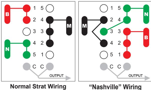
On the left is the straight-up Strat wiring we explored previously. On the right is "Nashville" wiring, which is a term that's typically reserved for Teles, but will work here too. Note the difference in position 3:
