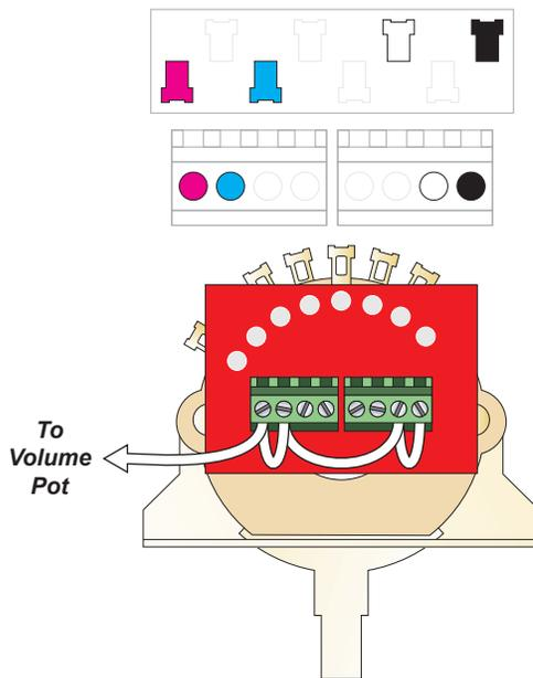
All three of these CORE switches are **2-pole** switches, meaning they're essentially two switches in one, though often you'll need both poles to accomplish an objective. Each pole has a **common** lug (CA & CB), that is connected to another lug in each switch position. In position 1 (the lever toward the rear of the guitar - bridge position) CA is connected to 1A, and CB is connected to 1B, like this:
