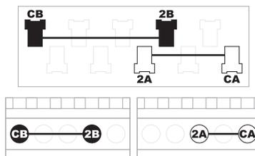
A couple of notes: The terminal blocks (the green things with the screws) are designed for stranded wire, not solid wire. They will work with thin solid wire (like the legs on a resistor), but thicker solid wire (like Orange Drop capacitor legs, or traditional treble bleed kits) aren't as well suited. For this reason we offer a range of accessories for this product line that have stranded wire leads.
