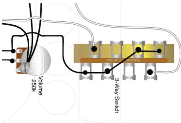
For example, in the crop above (from a Seymour Duncan diagram), four of the switch lugs are connected to each other, and then they connect to the input lug on the volume pot. Comparing this to our diagram (see above right), the four lugs in Duncan's diagram correspond to pink, blue, white, & black.
