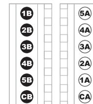
Our CORE components take the soldering out of your wiring situation, which makes it very straightforward to wire your guitar. The screw-down terminal blocks are easy to use. Just strip a little insulation from your wire, insert it into the appropriate slot, then tighten with the provided screwdriver. Easy and secure!
