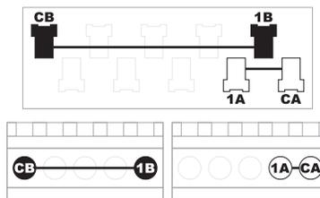
In position 2, the CA lug is connected to 2A, and CB is connected to 2B, and so forth.
