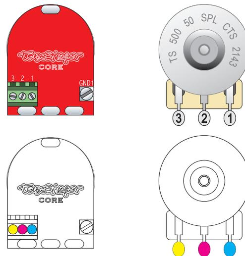
Our CORE pots couldn't be simpler. The terminal block has 3-2-1 references printed right on the board, and these map directly to the three pot lugs as shown at top. Below that is a color-coded version if you prefer it.
