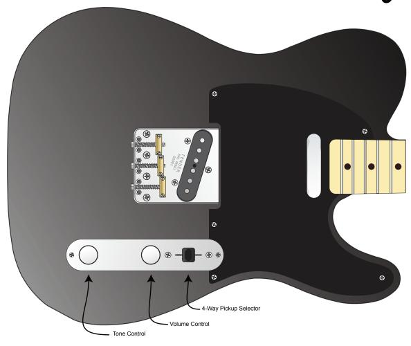
Wiring two coils together in series rather than parallel yields markedly different results. On Telecasters with 2 pickups, the traditional parallel wiring provides relatively consistent output across all three positions. A Telecaster with its pickups wired in series differs in that when both pickups are on at the same time, the combination produces higher output and a fatter tone. A 4-position Tele switch allows players to have both wiring options at once. The resulting pickup combinations are:
